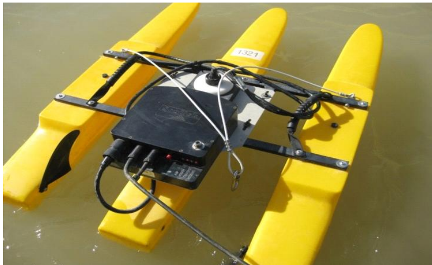
Fig. 3: SonTek River Surveyor ADCP
