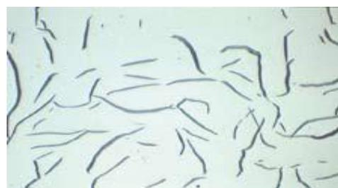
*Fig. 2: Well-polished graphite flakes*
