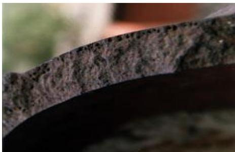
*Fig 3a. Gray surface after fracture*
