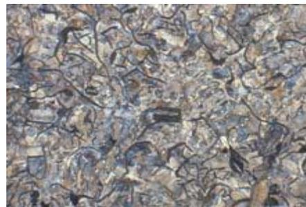
*Fig. 3b Grey iron with flake graphite in 200x pearlitic matrix*
