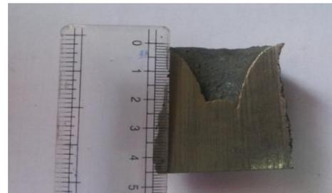
**Fig. photographs of Macro shrinkage of gray cast iron cylindrical height 23 cm & 17cm**
