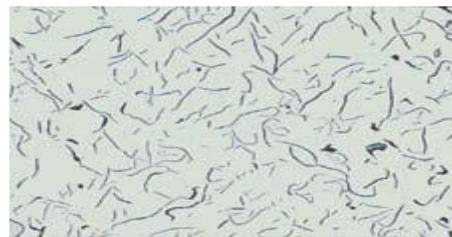
*Fig. 2: showing correct polish 200x*
